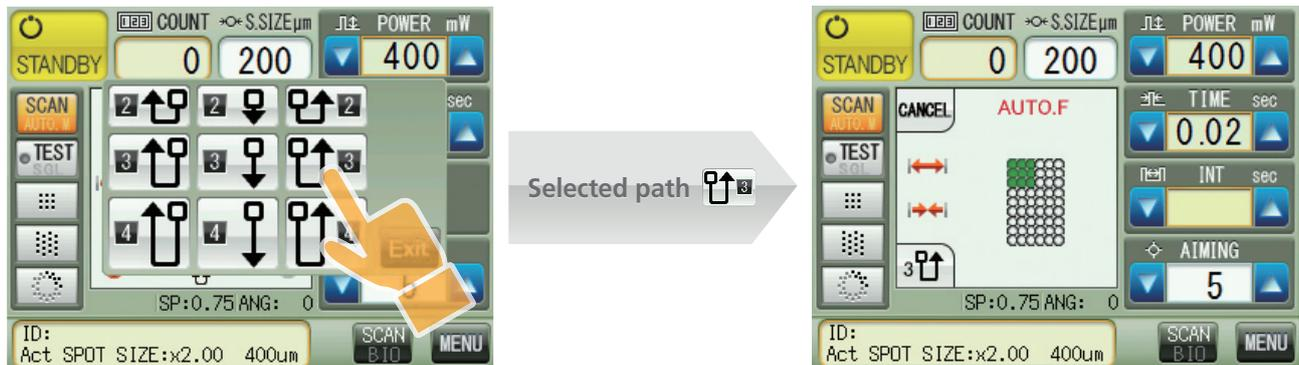
The repeat mode with the auto forward function enables consecutive regions to undergo photocoagulation on a selected path without repeatedly pressing the foot switch.
