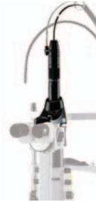
Attachable delivery unit (ZEISS SL-130, 30SL/M)
